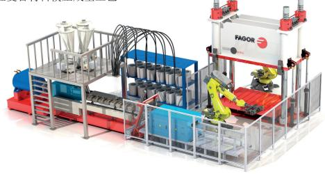
As this is a process where the thermoplastic matrix material is being compound in line, we offer the possibility to provide the whole process manufacturing equipment, from the compounder for raw material (pellets+fibers) to the final part unloading from the press, all full automatized. The type of extruder could also be different depending on customer needs.
