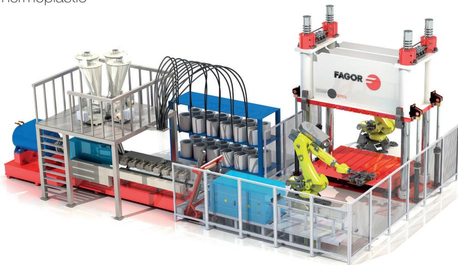
As this is a process where the thermoplastic matrix material is being compounded in line, we offer the possibility to provide the whole process manufacturing equipment, from the compounding for raw material (pallets + fiber) to the final part unloading from the press, all full automatized. The type of extruder could also be different depending on customer needs.
