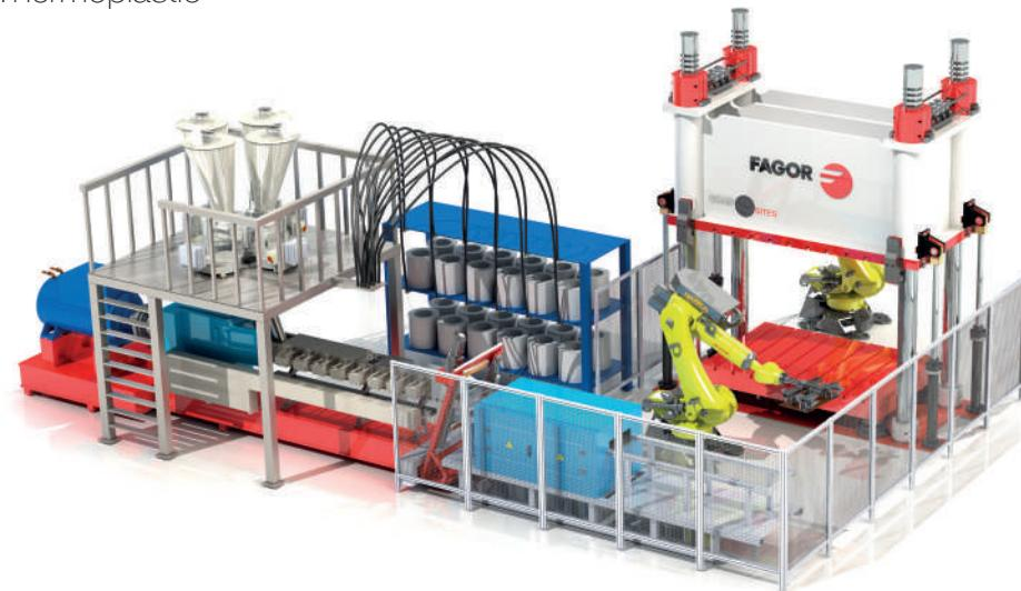
As this is a process where the thermoplastic matrix material is being compound in line, we offer the possibility to provide the whole process manufacturing equipment, from the compounder for raw material (pallets + fiber) to the final part unloading from the press, all full automated. The type of extruder could also be different depending on customer needs.
